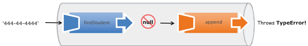
Figure 5.10 Functions findStudent and append are being composed. Without the proper checks, if the former produces a null return value, the latter will fail with a TypeError exception.
